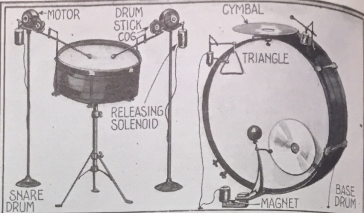
Solenoids and Magnets Control individual Strokes on the Bass Drum, Cymbal and Triangle, While a Motor-Driven Cog Causes the Rat-tat-tat of the Snare Drums.
