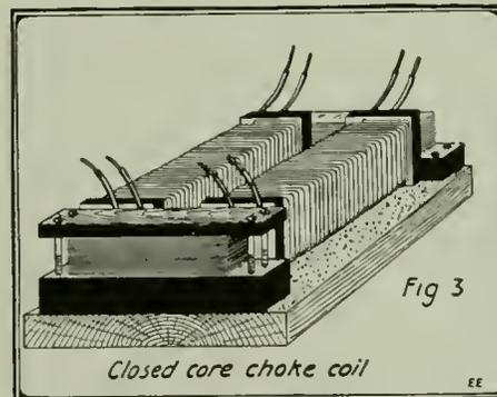
A Well-Designed Choke Coil of the Double-Pole, Closed-Core Type. One-half of the Winding Is Placed on Each Leg of the Laminated Sheet Iron Core.
