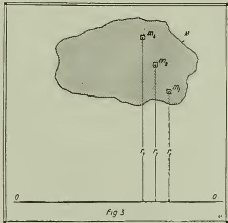
Fig. 3. Another Form of Expression for the Energy of a Rotating Body May Be Obtained by Determining Its Moment of Inertia. Here the Mass M is Subdivided Into Minute Parts  $m_1, m_2, m_3$ , etc. The Sum of the Products of These Masses and the Squares of Their Distances is the Moment of Inertia, Which with the Angular Speed, Gives the Kinetic Energy E.
