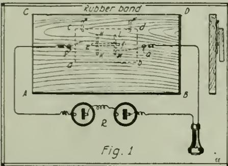
Here, ABCD = Piece of Soft Wood 5 x 3 x 1/4 inches Resting on Wooden Base. abcd = Wooden "Mouthpiece" Hanging on Back of Larger Piece and Carrying a Short Carbon Rod, ef. HK and LM = Carbon Rods Attached to the Larger Piece of Wood. Wires Lead from HK and LM Thru the Posts p and q and Two Dry Cells at R to the Standard 75 Ohm Telephone Receiver.
