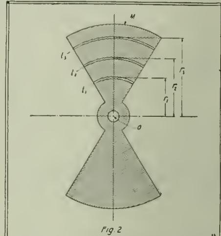
Fig. 2. In This Case the Mass M, Rotating  $n$  Times Per Second, About An Axis O, is Divided Into Numerous Elements or Small Parts at Various Radii from O. Knowing the Kinetic Energy of Each Part, the Whole Kinetic Energy of the Mass is Easily Determined by Taking a Summation of the Individual Quantities.
