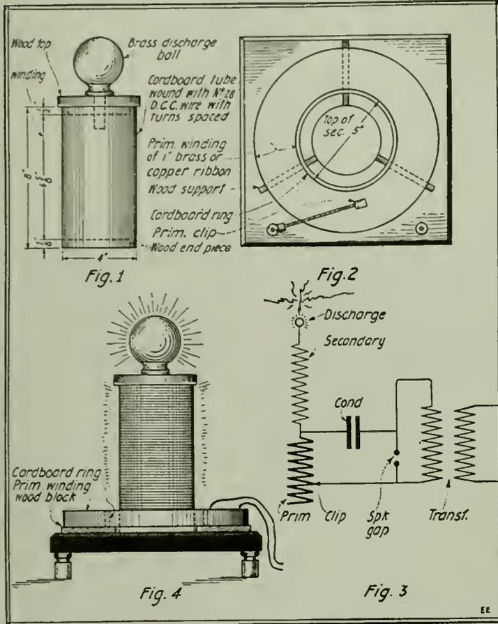
An 8- to 10-Inch Spark Oudin High Frequency Coll. It Can Be Excited by a One-quarter K. W. Step-up Radio Transformer or 6- to 8-Inch Spark Coll.
