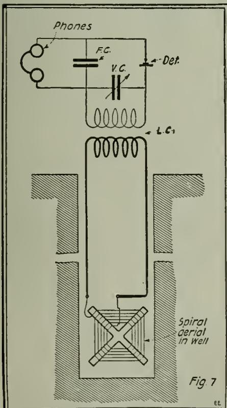
Some Very Surprising Results Were Obtained in Receiving with a Spiral Antenna Lowered into a Dry Well. Slightly Different Results Were Noticed with Water in the Well.
