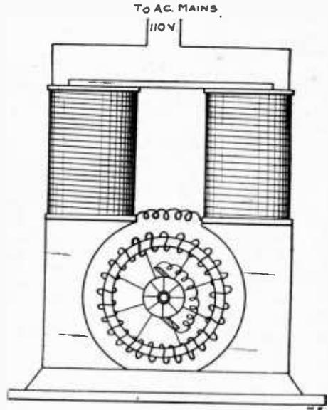
the position of the brushes, for in this way the speed of the motor and direction of rotation is controlled. At low speed this motor is very powerful, but as the speed increases the power decreases.
