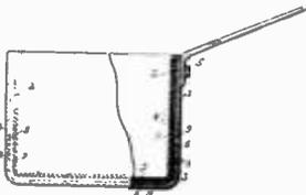
1. An electrically heated vessel which comprise, an inner shell, an outer coating of insulation for said shell, an outer shell in which said inner shell is set, said inner shell being spaced from said outer shell, an inner heat insulating lining for said outer shell and spaced from said inner shell, a heating coil wound around said inner shell within the space between the shells, and a cement filler in said space between said shells to unite the same and embed said heating coil.
