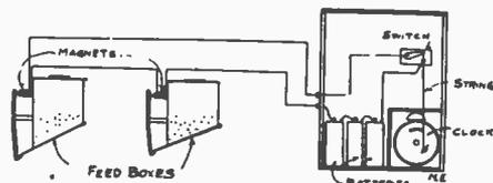
shown so that it can work freely. To the upper end is fastened a soft iron disc 1/2x1/8 inch, this is to act as armature. At the lower end is cut a notch for the bottom of the feed box to rest in. Note how the bottom is hinged so that when released it falls. The armature should be about 3/8 inch from the magnet core.
