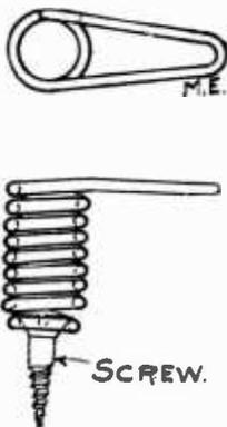
up No. 18 Phosphor Bronze or Brass Spring Wire on an one-eighth inch rod. The bottom coil is slightly bent to hold the No. 3 wood screw, and the top coil is bent as shown to form a small handle. By pressing this handle,
