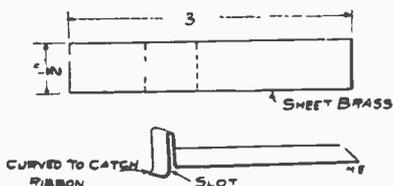
so as to make a slot for the ribbon to fit into. This will prove to be a very good clip and can easily be made by studying the drawing.
