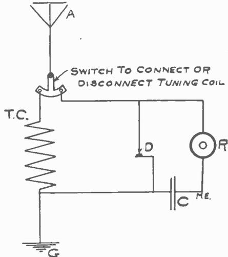
small case which contains the detector, and a condenser consisting of sheets of a tinfoil or copperfoil separated by some collodion, or better yet, "Healskin," and a switch. The cane does duty as both aerial and ground.
