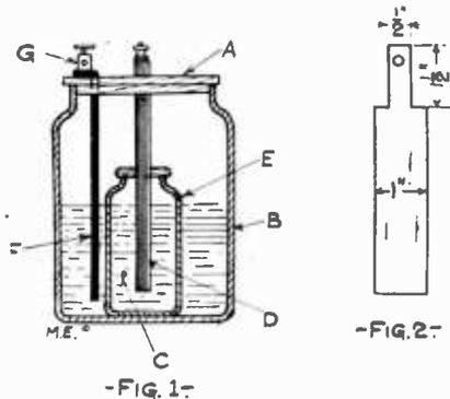
sulphuric acid. This style of interrupter has given the writer excellent results. Using 220 volts A. C., he was able to draw a spark an inch long from a coil whose secondary was composed of three quarters of a pound of No. 32 S.C.C. wire.
