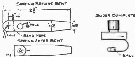
Use about No. 22 or No. 24 spring brass and one-quarter inch steel ball. The holes inside of spring strip where ball runs should be beveled smooth. The drawing explains the rest.
