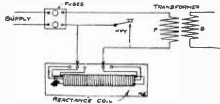
but not enough to cause a spark at the gap. Now when the key is pressed the full line current is allowed to flow through primary of transformer causing a spark to jump the gap.
