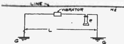
to rapidly make and break the circuit, to two ground terminals as shown, we can read any telegraph message which may be sent upon a line with a ground return, provided that the legs of the device are a sufficient distance apart. It was found on a small experimental line that, in general, a distance as small as about one-hundredth of the length of the
