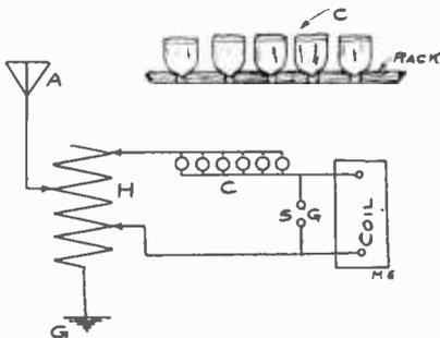
edged tool. Mount the globes on a frame after covering them with tinfoil.
