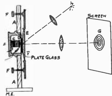
at G by reflection. Seeing that the distance between the line and the plate is quite small, it will be considerably changed by any movement of the telephone diaphragm. When a signal is received the rings on the screen will expand out or contract and also change color, so that this gives a good signal for the operator. Should it be desired to make a permanent record, a photographic paper band can be driven along back of the screen and light is let in
