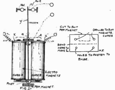
The instrument is now mounted on a base. This is done by fixing an angle-shaped piece of brass at A. See Fig. 2. The contact posts, and springs are placed as in Fig. 1. Contact No. 2 is tipped with platinum.
