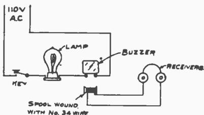
The sound may be regulated by moving the coil to or from the buzzer.
