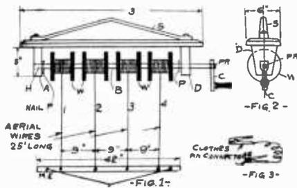
B, separated at a distance so as to let the four No. 14 B and S aluminum wires 25 feet long fall nine inches apart, as in Fig. 1. Mount this rod, B, on an axis, one end in the hole, H, and the other through the support, D, to a wooden crank, C, 8 inches long.
