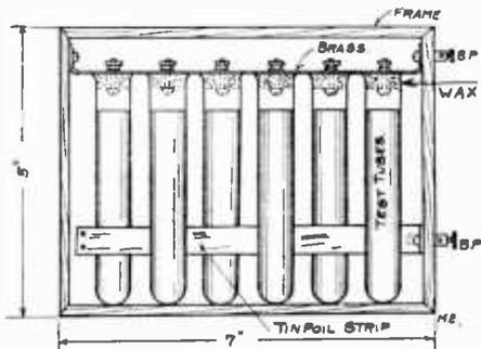
enough wax, taken from the top of the battery, to secure them in place. Paste tinfoil over the outer surface of tubes to within an inch of the top. Connect the binding-posts together by a strip of brass in which holes have been made at suitable intervals to screw the binding-posts into
