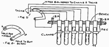
Solder wire onto chain and run from inside of one jar to one brass tack. Do the same with all the jars. Be sure to
