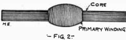
one layer of 50 turns of No. 16 D. C. wire over this. See Fig. 1. Then wrap a layer of cloth, which need not be shellacked because the whole transformer will be placed in oil, around this, then another of wire and cloth,
